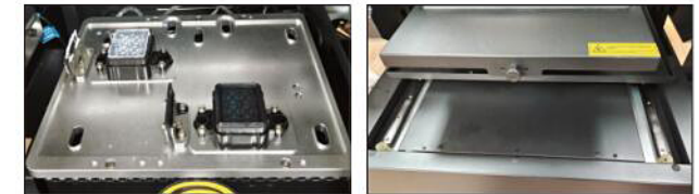
Liftable Capping Station
