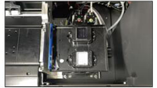
Lifting capping station
