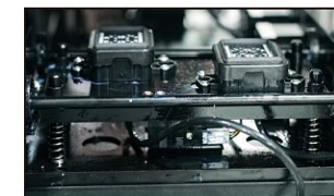
Lifting Capping Station
